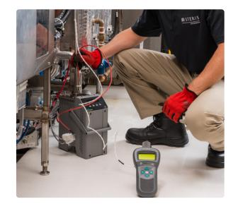
Calibration and verification points are determined by STERIS, the manufacturer or your SOPs. We will make necessary adjustments to 'out of tolerance' conditions we may find and include the results in your final report.
